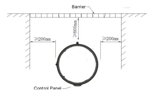
2. If heat pump installed in the basement, indoor or other airtight space, please note exhausting or intake circulation between surrounding air and outdoor air; The air duct total length should be equal or less than 6 meters, and the duct diameter should be equal or more than 150 mm.
