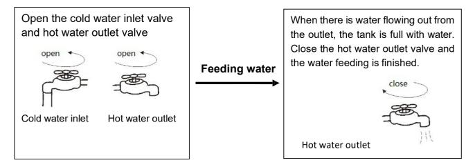
Operation without water in water tank may result in the damage of auxiliary E-heater. Due to such damage, manufacturer will not be liable for any damages caused by this issue.
