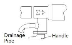
● Drainage pipe must be taken measures to keep temperature to prevent pipe from freezing to cause accident.
